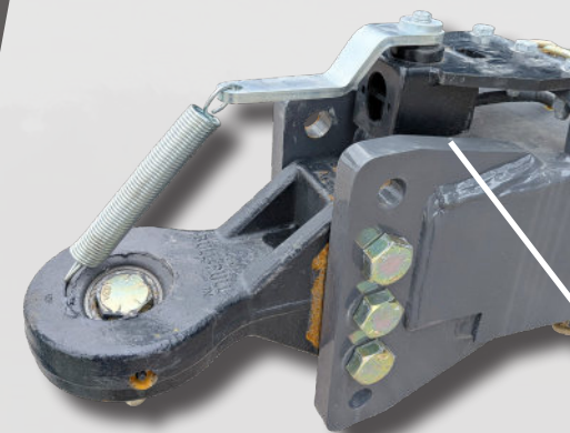
ANGLE TRANSDUCER BETWEEN TRACTOR AND IMPLEMENT
